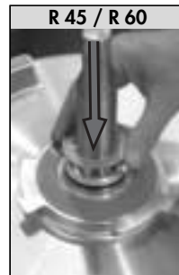
11) Place 1 mm thick washer
