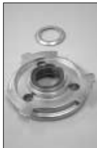
7) Socket and top seal are free
