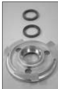
8) Replace shaft seals
