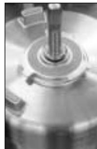
10) Replace shaft top seal, place it on shaft chamfer
